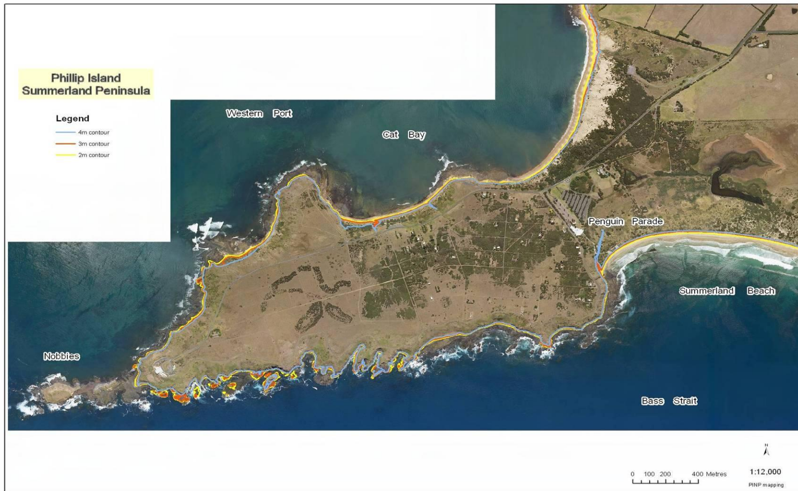
Figure 1.7. Mean sea-level contours for the Summerland Peninsula. Orange = current mean sea level, yellow = one metre rise (1 in a 100 year event currently), red = two metre rise, blue = three metre rise.
