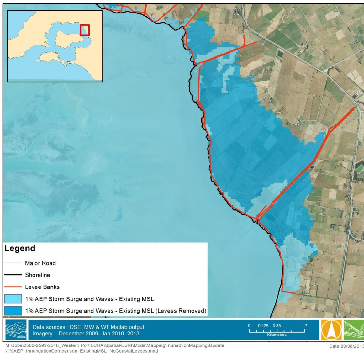
Figure 4-13 Estimates of Coastal Inundation under Existing Mean Sea Level Conditions with and without Informal Coastal Levees and Embankments
