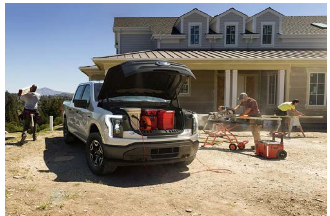
Figure 4 Vehicle to Load capabilities of the Ford F-150 Lightning
